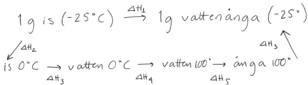
Hess lag:  $\Delta H_1 = \Delta H_2 + \Delta H_3 + \Delta H_4 + \Delta H_5 + \Delta H_6$
