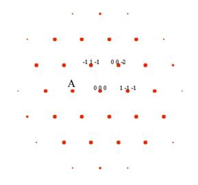
Fig. 1. Diffraction pattern from a gold crystal with the electron beam incident along the [110] direction.
