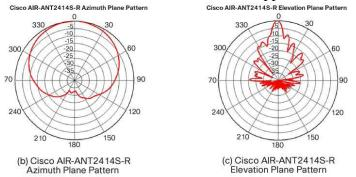
Assume that two identical base stations, each using these antennas, are placed perpendicular to each other in a shadowed urban environment. What is the minimum distance tolerated between the base stations if they should transmit in the same 5 MHz frequency band? Assume an output power of 10W and a receiver noise figure of 1.5 dB.
