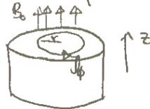
$$J_\phi(r, t) = \operatorname{Re} \{ J_\phi(r) e^{i\omega t} \} = \frac{6B_0 \omega r \sin(\omega t)}{2}$$
