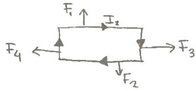
$$F_m = \frac{I_2 c \mu_0 I_1}{2\pi b} \hat{r} - \frac{I_2 c \mu_0 I_1}{2\pi a} \hat{r} \quad \text{At short sides the forces cancel each other.}$$
