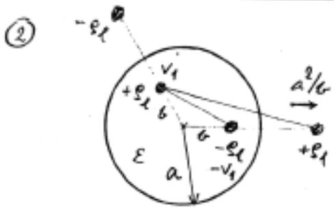
$$\begin{aligned} V_1 &= \frac{\rho_l}{2\pi\epsilon} \ln\left(\frac{a^2 - b^2}{r_0}\right) + \frac{\rho_l}{2\pi\epsilon} \ln\left(\frac{b\sqrt{3}}{\sqrt{b^2 + a^2/r_0^2 + a^2}}\right) \\ &= \frac{\rho_l}{2\pi\epsilon} \ln\left(\frac{(a^2 - b^2)b\sqrt{3}}{r_0\sqrt{a^4 + b^4 + a^2b^2}}\right) \end{aligned}$$
