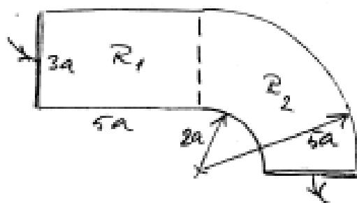
$$R_1 = \frac{1}{\sigma d} \cdot \frac{5a}{3a} = \frac{1}{\sigma d} \cdot \frac{5}{3}$$
