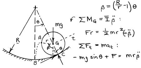
Eliminate F, substitute  $\beta = (\frac{R}{r} - 1) \theta$ ,  $\dot{\theta}$  assume Small  $\theta$ :  $\ddot{\theta} + \frac{29}{3(R-r)}\theta = 0$   $\omega_{\eta} = \sqrt{\frac{29}{3(R-r)}}, \quad \tau = \frac{2\pi}{\omega_{\eta}} = 2\pi\sqrt{\frac{3(R-r)}{29}}$
