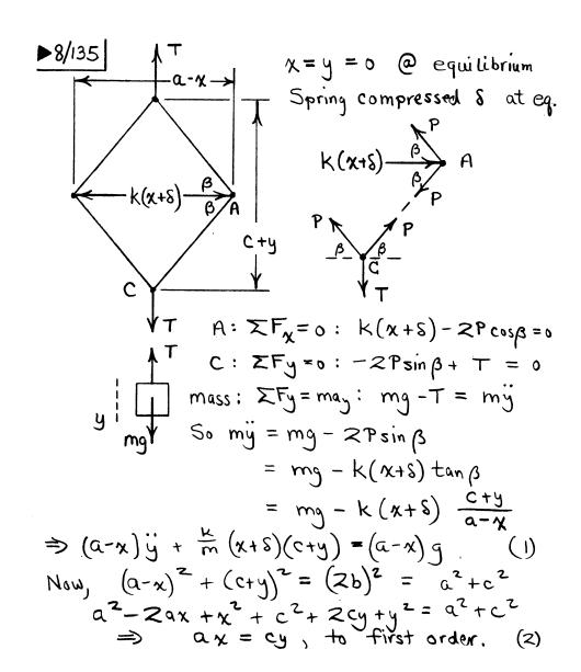
$$a\ddot{y} - x\ddot{y} + \frac{k}{m}cx + \frac{k}{m}cs + \frac{k}{m}xy + \frac{k}{m}sy = ag - xg$$
