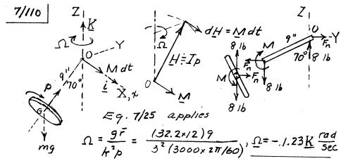
Results are independent of 70°-angle: (or  $\frac{1.23\times60}{2\pi}$  = 11.75 rev/min)  $M = I\Omega p \sin 70^\circ = mk^2 \left(\frac{g\bar{r}}{k^2p}\right) p \sin 70^\circ = mg\bar{r} \sin 70^\circ$ which agrees with static analysis of shaft where  $EM_0 = 0$  gives  $M = 8 \times 9 \sin 70^\circ$  M = 67.7i 16-in.
