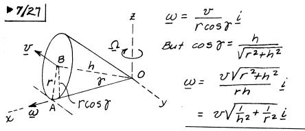
$$\omega = const \quad so \quad \alpha = \Omega \times \omega$$
