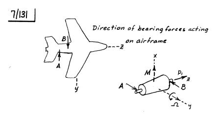
To satisfy  $M = I_{\underline{\Omega}} \times \underline{p}$   $p \text{ must be } \underline{p_i}$
