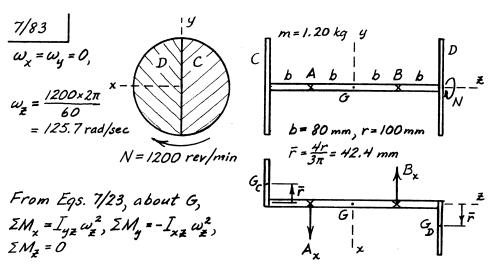
$$\begin{split} I_{yz} &= 0, \ I_{xz} = \left\{ 0 + m(2b)(\bar{r}) \right\} + \left\{ 0 + m(-2b)(-\bar{r}) \right\} = 4mb\bar{r} \\ &= 4(1.20)(0.080)(0.0424) = 0.01630 \ kg \cdot m^2 \\ \Sigma F_x &= 0 \ so \ A_x = B_x \\ \Sigma M_y &= -A_x b - B_x b = -4mb\bar{r} \, \omega_z^2, \ A_x = B_x = 2mb\bar{r} \, \omega_z^2/b \\ &\qquad \qquad A_x = B_x = \frac{1}{2} \left( 0.01630 \right) \left( 125.7 \right)^2 / 0.080 \\ &\qquad \qquad = 1608 \ N \end{split}$$
