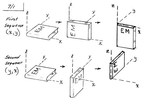
Final positions are different so finite rotations cannot be added as proper vectors
