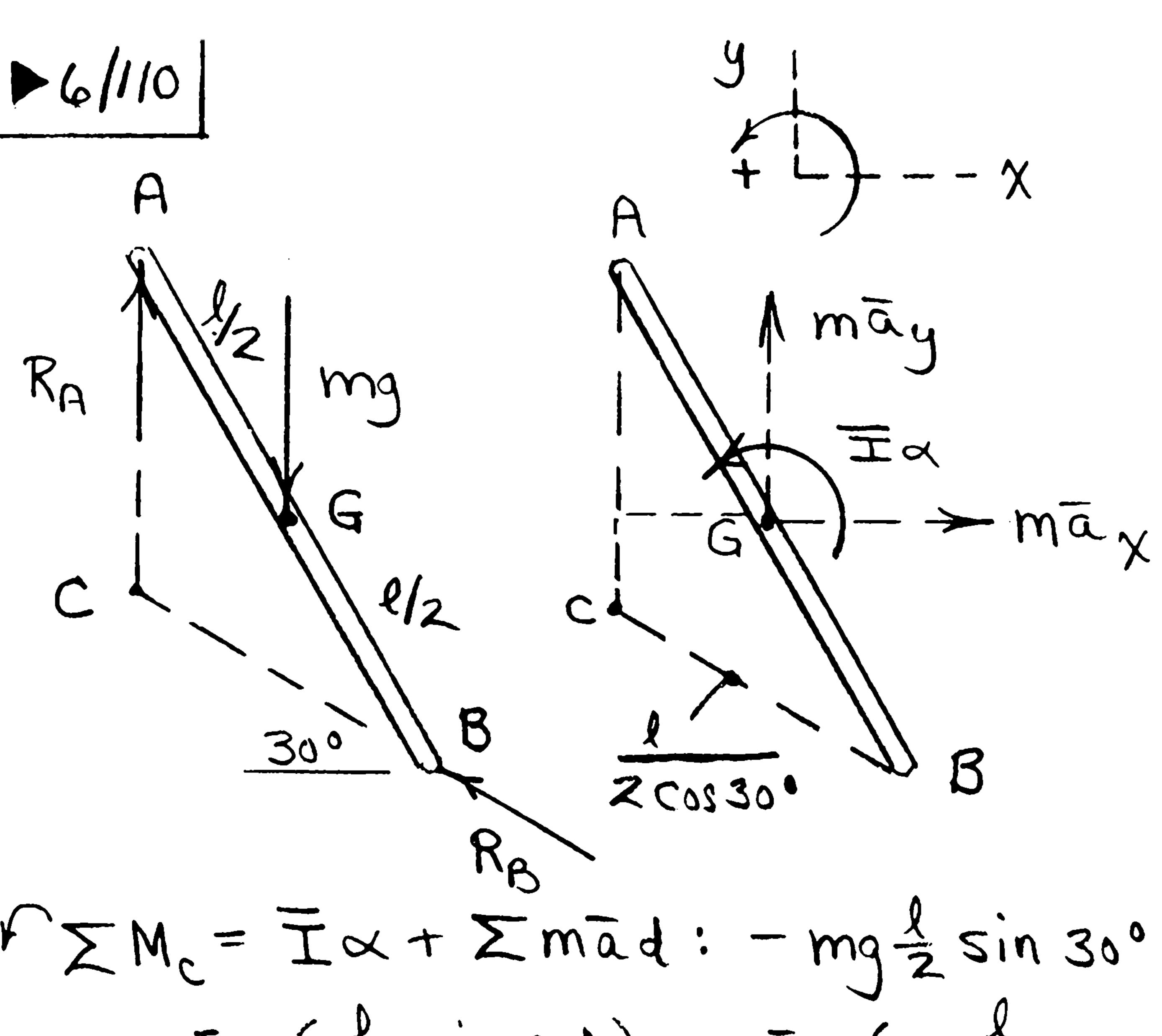
FIMC = IX+ Imad: - mg = sin 30° = 12ml2x + māy  $(\frac{1}{2}.5in 30^{\circ})$  - māx  $(\frac{1}{2 \cos 30^{\circ}} - \frac{1}{2} \cos 30^{\circ})$  (1)
