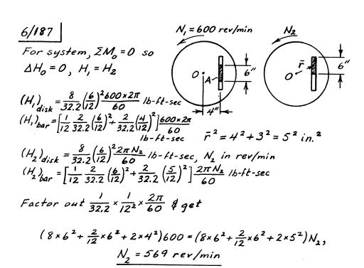
Friction forces in the slot are internal so have no effect on  $\mathbb{Z}M_0$ . Hence the final value of  $N_2$ , as well as the loss of energy, is unaffected.
