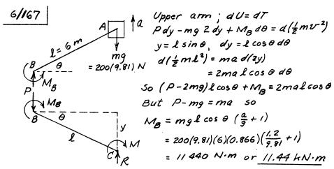
Lower arm; EM = 0;  $M + M_B - Pl. \cos \theta = 0$   $M = -mgl \cos \theta \left(\frac{\alpha}{g} + i\right) + mg\left(\frac{\alpha}{g} + i\right) l \cos \theta$ , M = 0M = 0 can be obtained by inspection since m is directly above C. Also, problem can be solved directly by  $F - m - \alpha$  equations.
