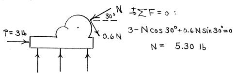
Wheel B:  $7 \times M_B = I_B \propto : 0.6(5.30)(\frac{10}{12}) = \frac{50}{32.2}(\frac{8}{12})^2 \propto$
