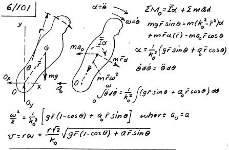
For  $\bar{r}=0.45m$ , r=0.8m,  $K_0=0.55m$ ,  $\Theta=45^\circ$ ,  $\alpha=109$ ,  $U = \frac{0.80\sqrt{2}}{0.55} \sqrt{9.81(0.45)(1-1/2)} + 10(9.81)(0.45) \frac{1}{12} = 11.73 \frac{m}{3}$ (Alternatively apply Eq. 6/3 with moment center at 0)
