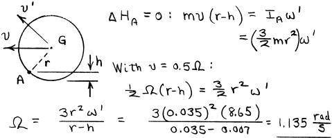
Neglect impulse of weight during import so that  $\Delta H_A = 0$ No that  $\Delta$
