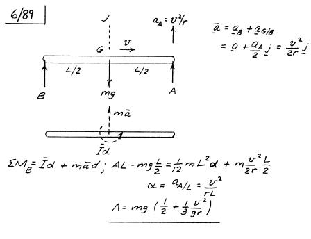
$$\sum M_{g} = \overline{I}d + m\overline{a}d; \quad AL - mg\frac{L}{2} = \frac{1}{12}mL^{2}d + m\frac{v^{2}L}{2}$$
