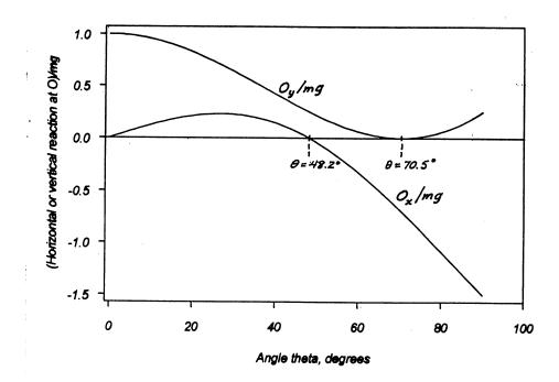
Increase in  $O_y$  from  $\theta = 70.5^{\circ}$  to  $\theta = 90^{\circ}$  reflects the fact that, in  $-\bar{a}_y = \bar{a}_n \cos\theta + \bar{a}_t \sin\theta$ ,  $\bar{a}_n \cos\theta$  is decreasing faster than  $\bar{a}_t \sin\theta$  is increasing, showing the effect of the multipliers  $\cos\theta$  and  $\sin\theta$  for  $\theta$  near  $90^{\circ}$ .
