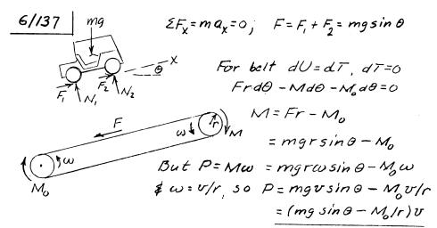
Static friction forces do positive work on belt and negative work on cart, both of equal magnitude
