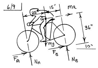
Tipping at front wheel:  $N_B$ ,  $F_B \rightarrow 0$   $+2 \times M_A = \text{mad}$ :  $mg (25 \cos 10^\circ - 36 \sin 10^\circ)$  = ma (36)Solve to obtain  $a = 0.510g (16.43 \text{ ft/sec}^2)$  6/10 As a whole:  $\Sigma F_{\chi} = ma: 80 = (6+4)q$ ,  $a = 8 m/s^2$
