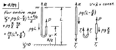
Entire rope:  $\Sigma F_{x} = G_{x}$ :  $R + P - pgL = \frac{d}{dt} \left( P_{z}^{x} v \right) = \frac{1}{2} \rho v^{2}$  --- (1) Work-energy:  $dU' = dT + dV_{g}$ :  $Pdx = d\left(\frac{1}{2} \rho \frac{x}{2} v^{2}\right) + d\left\{\frac{P_{z}^{g}(L^{2} + \frac{x^{2}}{2})}{2}\right\}$   $= \frac{1}{4} \rho v^{2} dx + \frac{1}{2} \rho gx dx$   $P = \frac{1}{4} \rho v^{2} + \frac{1}{2} \rho gx - \cdots (2)$ Sub. (2) into (1)  $R = \frac{1}{4} \rho v^{2} + \rho g(L - \frac{x}{2})$
