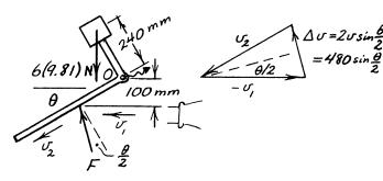
$F = m'\Delta \sigma$ :  $m' = pA\sigma = 1.206 \frac{\pi \times 0.040^2}{4} 240 = 0.364 \text{ kg/s}$
