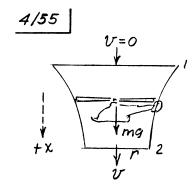
For system between sections 1 \$2  $\Sigma F_{x} = m' \Delta v_{x}$   $mg = \rho \pi r^{2} v(v-o)$   $v = \frac{1}{r} \sqrt{\frac{mg}{\pi \rho}}$
