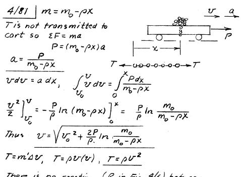
There is no reaction (R in Fig. 4/6) between departing links of cart, so mu is zero & EF=ma
