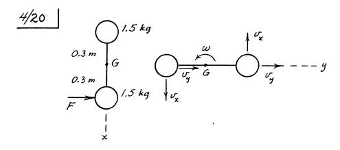
$$\begin{split} \sum E_{x} dt &= 0 \quad \text{so} \quad \Delta G_{x} = 0 \\ \sum E_{y} dt &= \Delta G_{y} \colon \ 10 = 2(1.5) v_{y} \,, \ v_{y} = 3.33 \,\text{m/s} \\ \sum M_{G} dt &= \Delta H_{G} \colon 10(0.3) = 2(1.5) v_{x}(0.3), \ v_{x} = 3.33 \,\text{m/s} \\ v &= 3.33 \sqrt{2} = 4.71 \,\text{m/s} \,\text{ both spheres} \end{split}$$
