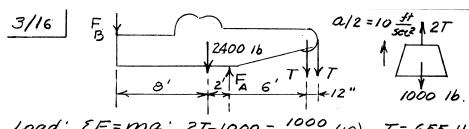
Load; EF = ma;  $2T - 1000 = \frac{1000}{32.2} (10)$ , T = 655 / 6Beam;  $EM_g = 0$ ;  $2400(8) - 10F_A + 655(16 + 17) = 0$  $F_A = \frac{4080 / 6}{10}$
