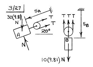
Kinematic constraint: L= 25A + 35B
