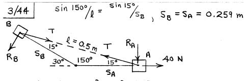
Law of cosines:  $l^2 = s_A^2 + s_B^2 - 2s_A s_B \cos 150^\circ$   $2ll = 0 = 2s_A v_A + 2s_B v_B - 2(-\frac{13}{2})(s_A v_B + s_B v_A)$  $s_A v_A + s_B v_B + \frac{\sqrt{3}}{2}(s_A v_B + v_A s_B) = 0^*$
