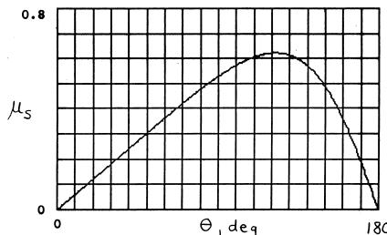
Note that it is impossible to see slippage  $\frac{\text{first}}{\text{greater}}$  occur at any angle greater than  $\theta = 121.9^{\circ}$ !
