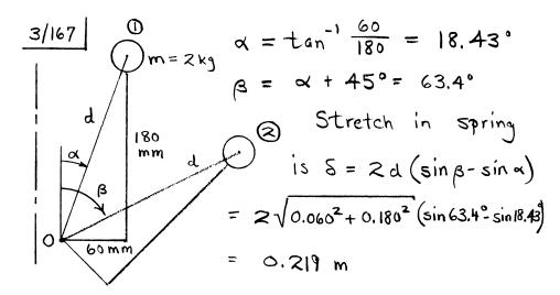
$T_1 + V_1 = T_2 + V_2$ , datum at 0  $0 + 2 mgd \cos \alpha = 0 + 2 mgd \cos \beta + \frac{1}{2} k S^2$   $2(2)(9.81)(0.1897)\cos 18.43° = 2(2)(9.81)(0.1897)\cos 63.4$  $+ \frac{1}{2}k(0.219)^2$
