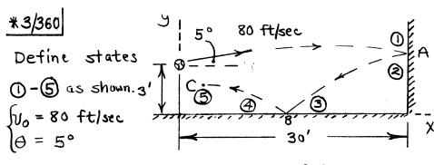
$$v_{0x} = v_0 \cos \theta = 80 \cos 5^\circ = 79.7 \text{ ft/sec}$$
