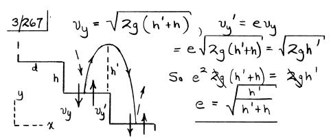
From y-displacement equation  $y=y_0+v_y_0t-\frac{1}{2}gt^2$ :  $-h=\sqrt{2gh'}t-\frac{1}{2}gt^2$ Solve for  $t=\sqrt{\frac{2}{g}}[h'\pm\sqrt{h'+h}]$ Choose (+) sign, as (-) sign yields t<0.
