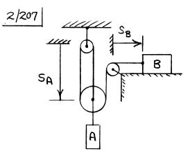
Length of cable  $L = S_B + 3S_A + \text{constants}$   $0 = U_B + 3U_A$ ,  $U_A = -\frac{U_B}{3} = -\left(\frac{-1.2}{3}\right) = 0.4 \frac{m}{s}$ (down)
